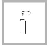
**4.** Add the contents of one NitraVer 5 Nitrate Reagent Powder Pillow (the prepared sample). Stopper.
