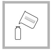
7. When the timer beeps, fill a second sample cell with 10 mL of sample (the blank). Place the blank into the cell holder.
