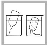
**3.** Collect at least 40 mL of sample in a 50-mL beaker. Fill a NitraVer 5 Nitrate AccuVac Ampul with sample. Place a stopper over the tip of the ampul.
