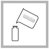
**3.** Fill a sample cell with 10 mL of sample.
