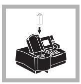
**9.** Place the prepared sample into the cell holder. Close the light shield. The result in mg/L nitrate nitrogen (NO<sub>3</sub><sup>-</sup>–N) will be displayed.
