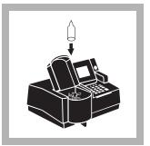
**10.** Place the AccuVac Ampul into the cell holder. Close the light shield. Results in mg/L nitrate expressed as nitrogen (NO<sub>3</sub><sup>-</sup>–N) will be displayed.
