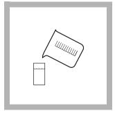
**6.** When the timer beeps, fill a zeroing vial (the blank) with at least 10 mL of sample.
