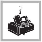
**8.** Place the blank into the cell holder. Close the light shield.
