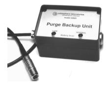
The green LED is on as long as the battery charge is OK. The red LED is on when charging is needed. To save batteries, both LEDs are out when the backup unit is in use, and mains power is out.
