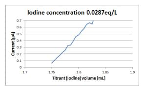
Titration with predose volume too high. No equivalent point will be found. The current at the beginning of the titration is not equal to 0 mA and it increases from the beginning of the addition.
