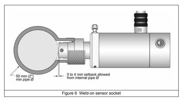
**Note:** Be sure to remove the two O-rings from the socket before welding. Leave the socket stainless steel cap screwed on during welding to prevent thread distortion.
