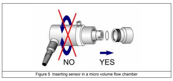
**Note:** Check that the small O-ring, located at the bottom of the micro volume flow chamber, is present during removal and installation of the sensor, as it may stick to the sensor head and fall.
