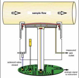
Figure 4 TC sensor working principle
