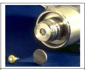
Thermal conductivity chip and membrane support
