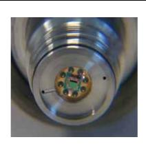
Thermal conductivity sensor cell with membrane and support removed
