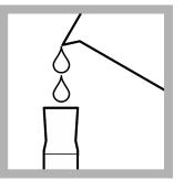
**3.** Use a graduated cylinder or pipet<sup>1</sup> to measure the sample volume from Table 1 on page 3.
