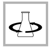
7. Swirl to mix. The addition of the powder pillow decreases the pH to 4 or less. If the sample has a high alkaline level, make sure that the solution pH is 4 or less before the next step.
