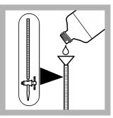
**2.** Fill a 25-mL buret to the zero mark with the titrant.
