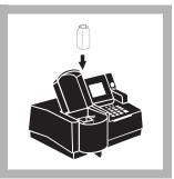
**7.** Place the prepared sample into the cell holder. Close the light shield. Read results in mg/L chlorine (or chosen units) within 1 minute of reagent addition.
