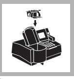
**3.** Insert the AccuVac Ampul Adapter into the sample cell module by sliding it under the thumb screw and into the alignment grooves. Fasten with the thumb screw.
