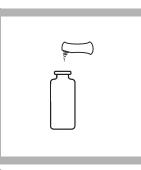
**6.** Add the contents of one DPD Free Chlorine Powder Pillow to the sample cell (the prepared sample). Swirl the sample cell for 20 seconds to mix. Proceed to Step 7 immediately.
