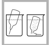
**7.** Fill a DPD Free Chlorine Reagent AccuVac Ampul with sample.
