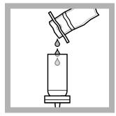
3. Pour or use a pipet to add the sample into the funnel. If the volume is less than 20 mL, add 10 mL of sterile buffered dilution water to the funnel.
