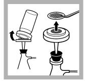
**6.** Stop the vacuum when the funnel is empty. Remove the funnel from the filter assembly. Use sterile forceps to lift the membrane filter.
