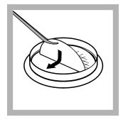
7. Put the membrane filter on the prepared agar plate. Let the membrane filter bend and fall equally across the agar to make sure that air bubbles are not caught below the filter.
