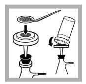
1. Set up the membrane filtration apparatus. Use a sterile forceps to put a membrane filter in the assembly. Make sure that the grid side is up.
