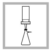
**4.** Apply the vacuum until the funnel is empty. Stop the vacuum.
