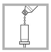
**5.** Rinse the funnel with 20 to 30-mL of sterile buffered dilution water. Apply the vacuum. Rinse the funnel two more times.
