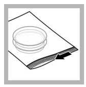
**9.** Put the inverted petri dish in a plastic bag and seal the bag.
