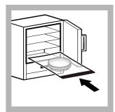
**10.** Incubate the inverted petri dish at the specified temperature for the specified time. Refer to Table 1 on page 3.
