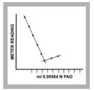
10. Draw the two best intersecting lines through the points as shown above. Find the volume of titrant to the nearest 0.01 mL at the intersection of the two lines. This is the mL titrant end point. This volume is equivalent to the free chlorine concentration in mg/L.
