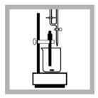
8. Continue the titration by recording at least three points on the downward sloping curve and at least three points after the end point has been reached. The value on the display will not change significantly after the end point.
