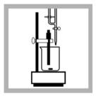
6. Dispense the titrant into the beaker in small increments while monitoring the values on the Amperometric Titrator. The values will decrease.
