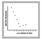
9. Make a graph of the titration. Plot the values from the amperometric titrator on the vertical axis and the corresponding volume of titrant on the horizontal axis.
