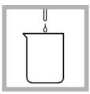
3. If the pH is less than 6 or greater than 7.5, add 1.0 mL of pH 7 Phosphate Buffer Solution to make the prepared sample.
