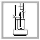
7. Continue dispensing slowly. Near the end point of the titration, write down the value on the display and the corresponding total volume of titrant that was added. Read the volume to the nearest 0.01 mL. Add a small amount of titrant and wait several seconds for a stable value. Write down the value.
