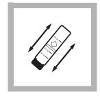
8. Remove the cap and add the contents of one BariVer Barium Reagent Powder Pillow to the sample cell. Tighten the cap on the cell and invert to mix.
