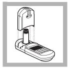
**6.** Put the sample cell in the cell holder. Put the instrument cap over the sample cell.
