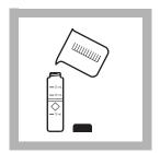
5. If the sample volume is less than 10 mL, add deionized water to the 10-mL line. Tighten the cap on the sample cell and invert to mix.
