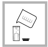
2. Prepare the blank: Rinse a 1-cm/10-mL sample cell and cap three times with sample. Fill the sample cell to the 5-mL mark with sample. Close the sample cell.
