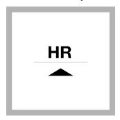
1. Set the instrument to high range (HR). For DR300, push the up arrow button. For PCII, push the menu button, checkmark button, then the menu button again.
