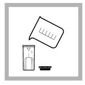
8. Prepare the sample: Rinse a second 1-cm/10-mL sample cell and cap three times with sample. Fill the sample cell to the 5-mL mark with sample.
