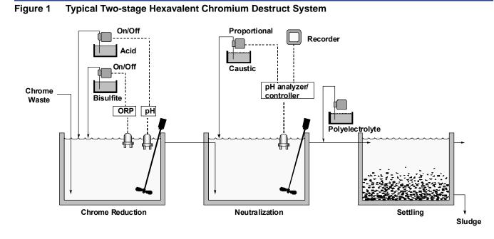
This reaction will progress rapidly between 2 and 3 pH. Retention time can be minimized by keeping the wastewater within this pH range. This is accomplished using a pH controller to add an acid such as sulphuric acid ( $H_2SO_4$ ).
