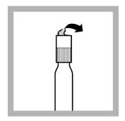
1. Carefully remove the foil from the screwed-on DosiCap Zip.
