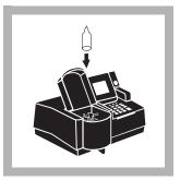
8. Immediately place the AccuVac Ampul into the vial adapter. Close the light shield. Result in μg/L dissolved oxygen (or chosen units) will be displayed.
