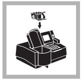
**3.** Insert the AccuVac Ampul Adapter into the sample cell module by sliding it under the thumb screw and into the alignment grooves. Fasten with the thumb screw.
