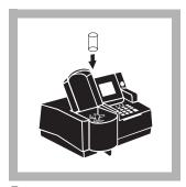
**5.** Place the blank into the cell holder. Close the light shield.
