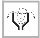
7. Fill a Low Range Dissolved Oxygen AccuVac Ampul with sample.
