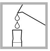
**4.** Use a graduated cylinder or pipet to measure the sample volume from Table 1 on page 3.
