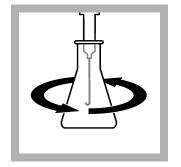
**9.** Put the end of the delivery tube fully into the solution. Swirl the flask. Turn the knob on the Digital Titrator to add titrant to the solution. Continue to swirl the flask. Add titrant until the color changes from yellow to light pink. Record the number of digits on the counter.
