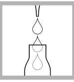
2. Carefully pipet 0.2 mL of solution A.
