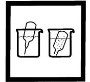
**5.** Fill a SulfaVer 4 Sulfate AccuVac ampul with sample.
