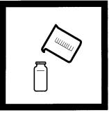
**3.** Stir the sample and immediately pour 25 mL of the blended sample into a sample cell (the prepared sample).
