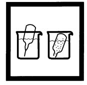
**6.** Fill a PhosVer 3 Phosphate AccuVac ampul with sample.
