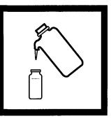
**4.** Fill a sample cell (the blank) with 25 mL of demineralized water.
