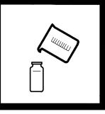
**8.** Pour 25 mL of sample (the blank) into a sample cell.
