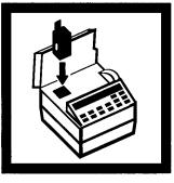
**8.** Place the AccuVac Vial Adapter into the cell holder.
