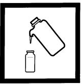
**6.** Fill a second cell with 25 mL of colorless water (the blank).
