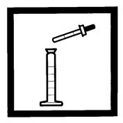
**5.** Add 1 mL of Molybdate Reagent using a 1–mL calibrated dropper.
