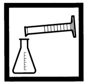
**4.** Measure 100 mL of demineralized water into a 500-mL erlenmeyer flask (the blank).
