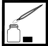
**2.** Remove the cap from the Bactrol inoculum bottle. Pick out one Bactrol Inoculum Disk with the sterilized forceps.
