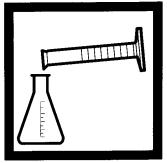
**5.** Measure 100 mL of sample into a second 500–mL erlenmeyer flask (the prepared sample).
