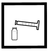
**8.** Pour the portion remaining in the cylinder into a second sample cell (the prepared sample).
