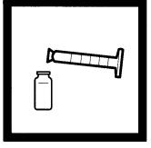
**8.** Pour the solution from the cylinder into a sample cell (the prepared sample).
