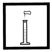
**5.** Add the contents of one ZincoVer 5 Reagent Powder Pillow. Stopper. Invert several times to completely dissolve powder.
