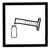
**5.** Fill a second sample cell (the prepared sample) with 25 mL of sample with a 25–mL graduated cylinder.
