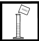
**3.** Measure 300 mL of sample in a 500–mL graduated cylinder.
