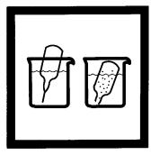
**5.** Fill a High Range Dissolved Oxygen AccuVac Ampul with sample.
