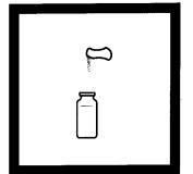
**9.** When the timer beeps, add the contents of one Amino Acid F Reagent Powder Pillow to one of the sample cell. Swirl to mix. This is the prepared sample.
