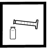
7. Pour 25 mL of the mixture into a sample cell (the blank). Add the contents of one Thiosulfate Powder Pillow to the sample cell. Swirl for 30 seconds to mix.
