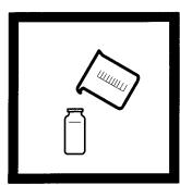
7. Pour 25 mL of sample into another sample cell. Immediately place this sample cell into the cell holder. Close the light shield.
