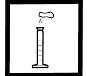
**5.** Add the contents of one Silver 2 Reagent Solution Pillow to the cylinder. Swirl to completely wet the powder.
