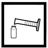
**4.** Fill a sample cell (the blank) with 25 mL of demineralized water with a 25–mL graduated cylinder.
