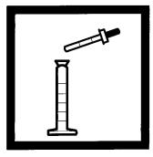
**6.** Add 1 mL of Amino Acid Reagent Solution. Stopper and invert several times to mix (the prepared sample).
