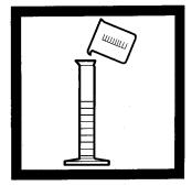
**1.** Measure 300 mL of demineralized water in a 500–mL graduated cylinder.
