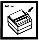
2. Rotate the wavelength dial until the small display shows: 605 nm
