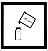
7. When the timer beeps, the display will show:  $mg/l O_3 DPD$ Fill a second sample cell (the blank) with 25 mL of sample. Place it into the cell holder. Close the light shield.
