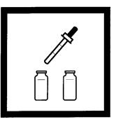
**7.** Add 1.0 mL of Sulfide 2 Reagent to each cell. Immediately swirl to mix.
