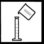
**4.** Fill a 25–mL graduated mixing cylinder with 25 mL of sample.
