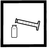
**11.** Pour the prepared sample into a sample cell. Place the prepared sample into the cell holder. Close the light shield.
