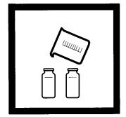
**4.** Fill two sample cells to the 25–mL line with sample.
