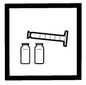
**5.** Split the diluted sample by pouring 25 mL into each of two sample cells.
