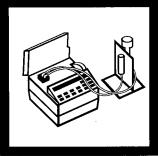
**4.** Install the Pour–Thru Cell and flush with 50 mL of demineralized water.
