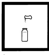
**6.** Add the contents of one Potassium Persulfate for Phosphonate Powder Pillow to one of the two sample cells. Swirl to mix. This sample cell contains the prepared sample.
