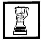
**1.** Homogenize 500 mL of sample for 2 minutes in a blender.
