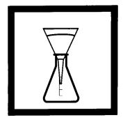
**5.** Filter or centrifuge 25 mL of the sample using labware listed under *Required Apparatus*.
