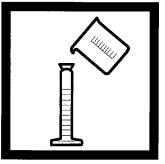
**4.** Fill a 50–mL graduated mixing cylinder to the 50–mL mark with sample.
