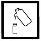
**4.** Fill a clean sample cell to the 25–mL mark with demineralized water (the blank).
