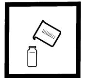
**5.** Fill another sample cell (the prepared sample) with 25 mL of sample.
