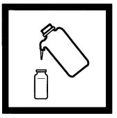
**4.** Pour 25 mL of demineralized water (the blank) into a sample cell.
