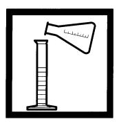
**6.** Fill a clean 50–mL plastic graduated mixing cylinder with sample from one of the flasks and then discard the cylinder contents.
