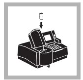
**20.** Place the Control into the adapter and close the light shield. Record the absorbance value of the Control.
