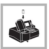
**18.** After the absorbance of the Control has decreased to  $0.60 \pm 0.10$  abs., place the Blank into the adapter and close the light shield.
