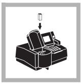
**15.** Place the Control into the adapter. Close the light shield. Record the absorbance.
