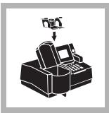
**4.** Insert the COD sample cell adapter into the sample cell compartment.
