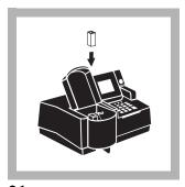
**21.** Place each sample or dilution into the adapter and close the light shield. Record each absorbance value.
