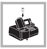
**6.** Place the blank into the cell adapter. Close the light shield.
