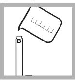
**5.** Fill a Test 'N Tube sample cell with deionized water. This is the blank.
