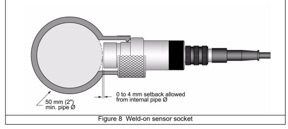
**Note:** Be sure to remove the two O-rings from the socket before welding and leave the sensor's stainless steel cap screwed on during welding to prevent thread distortion.
