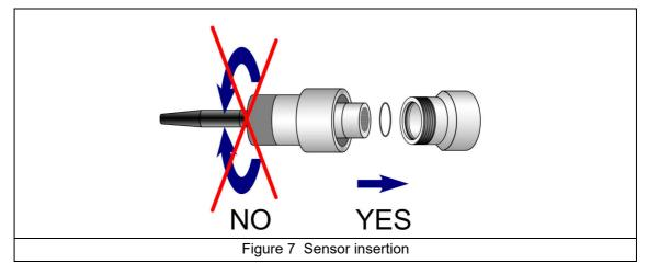
Note: Do not twist the sensor when inserting it into a micro volume flow chamber.
