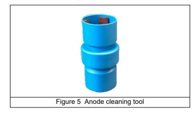
The blue anode cleaning tool (Figure 5) is used to clean the anode of any deposits or residue that may have formed. It is doubled-ended so it can be used for two membrane replacement processes, each end being used once.
