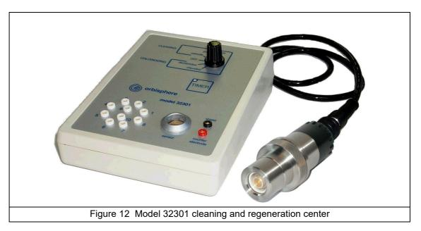
Use of this tool is recommended for a noticeably extended sensor life. Detailed information on how to use the cleaning and regeneration center is included in the 32301 Operator Manual.
