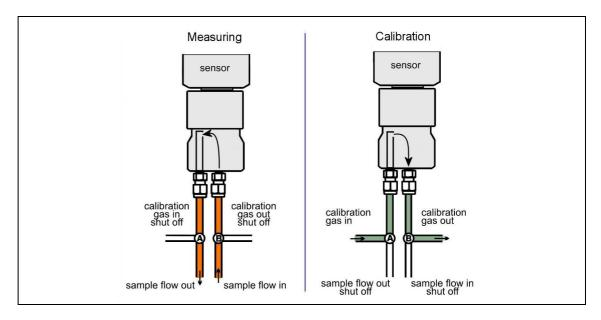
The manufacturer recommends to calibrate the Orbisphere ozone sensor at six months intervals and the internal pressure sensor of the analyzer at one year intervals. Do sensor maintenance before sensor calibration. Refer to 6.1 Maintenance on page 25.
