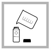
8. Prepare the sample: Rinse a second sample cell and cap three times with sample. Fill the sample cell to the 10-mL mark with sample.
