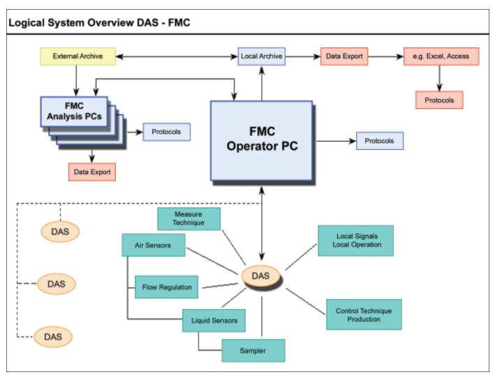
Figure 2. Overview of DigiPlan FMC-DAS software architecture.
