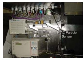
Figure 3. Instrumentation panel with HIAC HRLD sensor.
