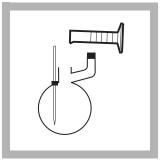
**8.** Add 25 mL of Hydrochloric Acid, ACS, to the distillation flask using a graduated cylinder.
