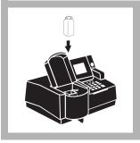
21. Place the reacted sample into the cell holder. Close the light shield. Results in mg/L arsenic (or chosen units) will be displayed.
