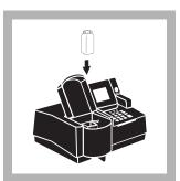
**18.** Place the blank into the cell holder. Close the light shield.
