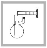
**6.** Measure 250 mL of sample into the distillation flask using a graduated cylinder.
