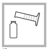
**17.** Fill a dry sample cell with unreacted arsenic absorber solution (the blank). Stopper. Place it into the cell holder.
