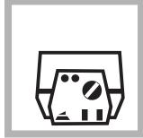
**7.** Turn on the power switch. Set the stir control to 5. Set the heat control to 0.
