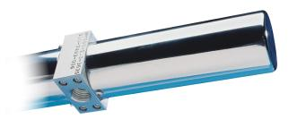
The HIAC HRLD Series light obscuration liquid particle counting sensors use laser diode technology to measure particles from 1.3 to 600 microns in a variety of fluids. For particles of 1.3 microns and larger, light obscuration is the preferred technology.
