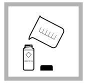
8. Prepare the blank: Rinse a sample cell and cap three times with sample. Fill the sample cell to the 10-mL mark with sample. Close the sample cell.
