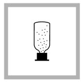
4. Hold the AccuVac Ampul with the tip down. Immediately put the stopper on the tip. The stopper prevents contamination from atmospheric oxygen.
