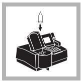
11. Place the AccuVac Ampul into the cell holder. Close the light shield. Wait approximately 30 seconds for the air bubbles to disperse from the light path. Results in mg/L (or chosen units) dissolved oxygen will be displayed.
