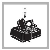
**9.** Place the blank into the cell holder. Close the light shield.
