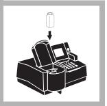
**7.** Place the prepared sample into the cell holder. Close the light shield. The results in mg/L ClO<sub>2</sub> (or chosen units) will be displayed.
