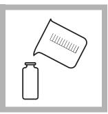
**6.** Fill another sample cell to the 10-mL mark with sample (the prepared sample).
