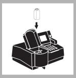
**12.** Place the prepared sample into the cell holder. Close the light shield. Results in platinum-cobalt units will be displayed.
