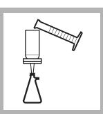
**3.** Rinse the filter by pouring about 50 mL of deionized water through the filter. Discard the rinse water.
