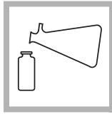
**9.** Fill a second sample cell (the prepared sample) with 10 mL of filtered sample.
