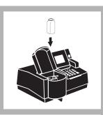
**10.** Place the blank into the cell holder and close the light shield.
