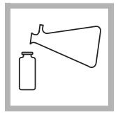
**5.** Fill a sample cell (the blank) with 10 mL of filtered deionized water. Discard the excess water in the flask.
