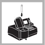
**10.** Place the sample vial in the cell holder and close the light shield.
