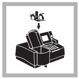
**8.** Insert the Test Tube Adapter into the sample cell module by sliding it under the thumb screw and into the alignment grooves. Fasten with the thumb screw.
