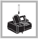
**16.** Place the prepared sample vial into the cell holder and close the light shield. Results in mg/L  $PO_4^{3-}$  (or chosen units) will be displayed.
