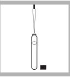
7. Using a TenSette Pipet, add 2 mL of 1.00 N Sodium Hydroxide to the vial. Cap tightly and shake to mix.
