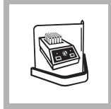
**1.** Turn on the COD Reactor. Heat to 150 °C. Place the plastic shield in front of the reactor.
