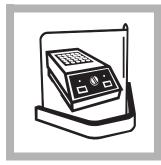
**5.** Place the vial in the COD Reactor, and start a 30-minute heating period by pressing the soft key under *START TIMER*.
