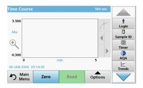
After all scan parameters have been selected, the instrument must then be zeroed. Afterward the sample can be analyzed.
