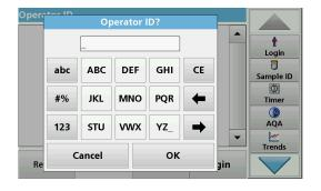
This display is used to enter letters, numbers and symbols as needed when programming the instrument. Unavailable options are disabled (grayed out). The icons on the right and left of the screen are described in Table 2.
