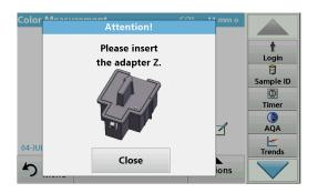
To use the 10 mm square cuvette and 11 mm round cuvettes, adapter Z must be inserted into the cuvette compartment (2). For measurements with 50 mm square cuvettes, you must remove the adapter.
