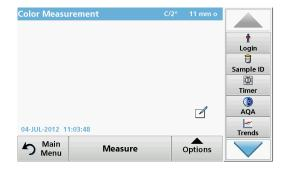
**4.** After calibration, the cuvette size used is displayed in the top right.
