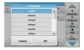
The software supports multiple languages. The first time the instrument is switched on, the language selection screen will be shown automatically after the startup process.
