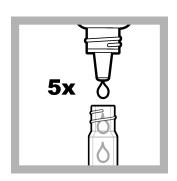
Immediately add 5 drops of Fluorescence Sulfite Reagent 2. Hold the bottle vertically.
