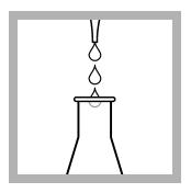
**15.** Add 2 mL of Starch Indicator Solution. A dark blue color develops.
