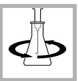
**12.** Put the delivery tube point fully into the solution and swirl the flask. Turn the knob on the Digital Titrator to add titrant to the solution. Continue to swirl the flask and add titrant until the color changes yellow to a pale yellow.
