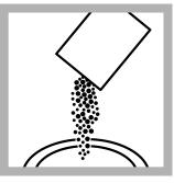
6. Remove the stopper and add the contents of one Sulfamic Acid Powder Pillow to the sample.
