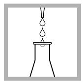
**13.** Add 2 mL of Starch Indicator Solution. A dark blue color develops.
