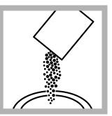
2. Add the contents of one Manganous Sulfate Powder Pillow and one Alkaline Iodide-Azide Reagent Powder Pillow to the sample.
