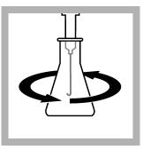
**16.** Put the delivery tube point fully into the solution and swirl the flask. Turn the knob on the Digital Titrator to add titrant to the solution. Continue to swirl the flask and add titrant until the color changes from a dark blue to a colorless end point. Record the number of digits on the counter.
