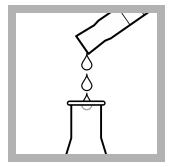
**9.** Accurately measure 20 mL of the prepared sample and transfer it to a 50-mL Erlenmeyer flask.
