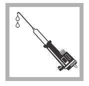
**11.** Hold the Digital Titrator vertically with the cartridge tip up. Turn the delivery knob to eject air and a few drops of titrant. Reset the counter to zero and clean the tip.
