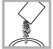
**6.** Remove the stopper and add the contents of one Dissolved Oxygen 3 Powder Pillow to the sample.
