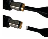
Once the sensor spot is removed do not touch the inside of the sensor as this could scratch and damage the exposed sensitive measuring head (indicated with arrow).
