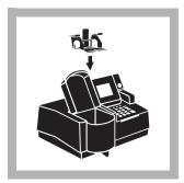
13. Insert the Test Tube Adapter into the sample cell module by sliding it under the thumb screw and into the alignment grooves. Fasten with the thumb screw.
