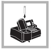
**16.** Place the prepared sample into the cell holder and close the light shield. The result in mg/L total inorganic nitrogen as nitrogen (N) (or chosen units) will be displayed.
