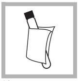
**14.** When the timer beeps, clean the outside of the vials with a towel, and place the blank into the cell holder.
