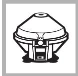
**7.** Centrifuge vials for 3 minutes or wait until solids settle to bottom of vial. Press the soft key under **START TIMER** to start a 3-minute period.
