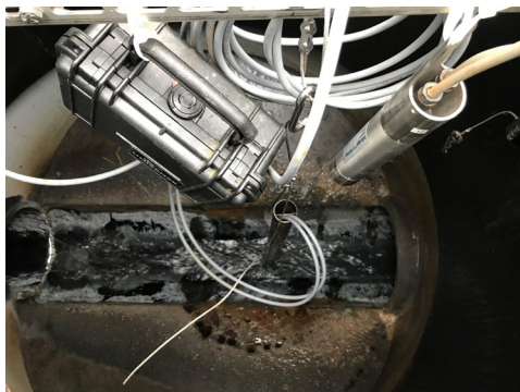
The Hach H 2 S sensor measures H 2 S directly in wastewater and in the air above.
