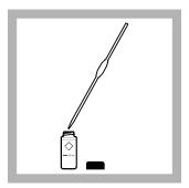
3. Prepare the sample: Use a pipet to add 10.0 mL of sample to a dry sample cell.
