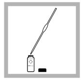
**4.** Use a pipet to add 2.0 mL of SPADNS or SPADNS2 Reagent Solution to each sample cell.
