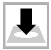
**8.** Insert the blank into the cell holder. Point the diamond mark on the sample cell toward the keypad.
