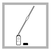
2. Prepare the blank: Use a pipet to add 10.0 mL of deionized water to a dry sample cell.
