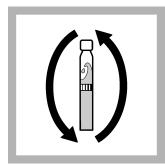
5. Blank-vial and Samplevial: Invert to mix.
