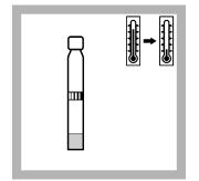
**9. Blank-vial and Samplevial:** Allow to cool down to room temperature in a cooling rack.
