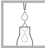
2. Blank-vial: Carefully pipet 2.0 mL of deionized water (blank). (Only 1 blank per batch)
