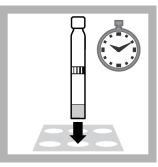
6. Blank-vial and Samplevial:. Heat in the reactor for 2 hours at 150 °C (302 °F).
