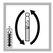
8. Blank-vial and Samplevial: remove the hot vials. Carefully invert twice.
