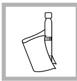
**10. Blank-vial and Sample-vial:** Thoroughly clean the outside of the vials.
