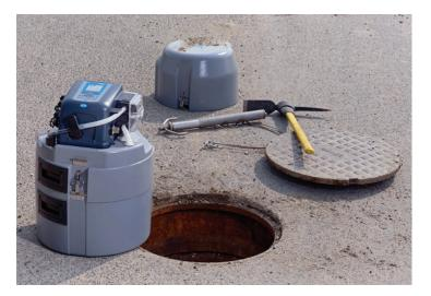
**Figure 2.** Using automatic samplers to collect multiple grab samples into a composite sample for every-other-day onsite testing improves the University of Denver's ability to identify SARS-CoV-2 viral presence in time to suppress COVID-19 outbreaks on campus.
