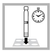
7. Place the vial into the **preheated** reactor. Heat in the reactor for **2 hours**.
