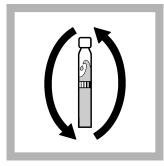
**2.** Invert a few times to bring the sediment into suspension.
