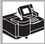
**23.** Close the light shield. The result in mg/L Free Ammonia as Nitrogen (NH<sub>3</sub>–N) will be displayed.
