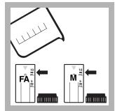
**4.** Fill two 10-mL/1-cm cells to the 10-mL line with sample.
