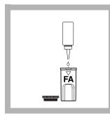
**9.** Add one drop of Free Ammonia Reagent Solution to the cell for Free Ammonia measurement.
