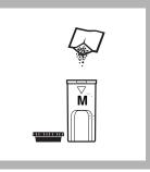
**7.** Add the contents of one Monochlor F pillow to the cell for the Monochloramine measurement.
