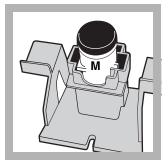
**13.** After the timer expires, place the Monochloramine cell into the cell holder so the locking ridge on the cell is oriented to the left. Press the top rim of the cell on the right side to lock it in place.
