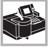
**14.** Close the light shield and read the result. The result in mg/L
