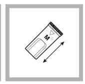
**8.** Cap the cell and shake for 20 seconds to dissolve the reagent.
