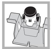
**5.** Place the Monochloramine cell into the cell holder so that the locking ridge on the cell is oriented to the left. Press the top rim of the cell on the right side to lock it in place. Close the light shield.
