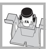
**22.** After the timer expires, place the Free Ammonia cell into the cell holder so the locking ridge on the cell is oriented to the left. Press the top rim of the cell on the right side to lock it in place.
