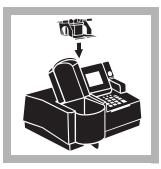
**3.** Insert the AccuVac<sup>®</sup> adapter into the sample cell module by sliding it under the thumbscrew and into the alignment grooves. Fasten with the thumbscrew.
