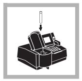
11. Place the prepared sample into the cell holder and close the light shield. The result in mg/L ammonia nitrogen (or chosen units) will be displayed.
