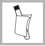
**9.** When the timer beeps, clean the outside of the vial with a towel, and place the blank into the cell holder. Close the light shield.
