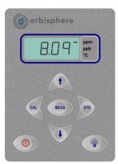
The button in the bottom right corner backlights the LCD for approximately three minutes. The other push-button controls are:
