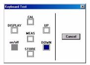
Press any one of the instrument's buttons (except the on/off button) for a full second or more. The appropriate square on-screen should darken.
