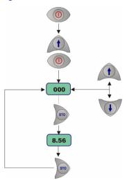
Switch the instrument **OFF** (by pressing the **POWER** key). Hold down the **1** button while switching the instrument back **ON**. The LCD displays a sample location number.
