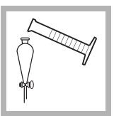
**3.** Measure 300 mL of sample in a 500-mL graduated cylinder. Pour into a 500-mL separatory funnel.
