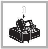
**15.** Place the prepared sample into the cell holder. Close the light shield. The result in mg/L nickel (or chosen units) will be displayed.
