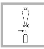
**11.** When the timer beeps wait for the layers to separate. Insert a peasized cotton plug into the delivery tube of the funnel. Drain the chloroform layer (bottom layer) into a sample cell (the prepared sample). Stopper.
