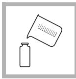
**13.** Fill a second cell (the blank) with 25 mL of chloroform. Stopper. Place the blank into the cell holder. Close the light shield.
