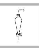
**6.** When the timer beeps, add the contents of one Nickel 2 Reagent Powder Pillow to the funnel. Stopper. Shake to mix.
