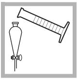
**8.** When the timer beeps, add 10 mL of chloroform. Stopper. Shake gently. Invert. With tip pointed up and away from people, open the stopcock to vent.
