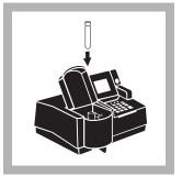
**16.** Place the prepared sample vial into the cell holder and close the light shield. Results in mg/L PO<sub>4</sub><sup>3-</sup> (or chosen units) will be displayed.
