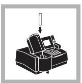
**14.** When the timer sounds, place the blank vial in the cell holder and close the light shield.
