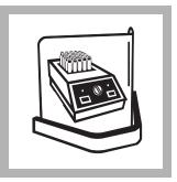
**7.** Place the vials in the COD Reactor, and start a 30-minute heating period by pressing the soft key under **START TIMER**.
