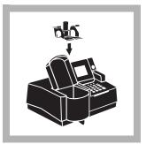
12. Insert the Test Tube Adapter into the sample cell module by sliding it under the thumb screw and into the alignment grooves. Fasten with the thumb screw.
