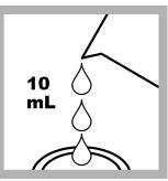
**6. Prepare the blank:** Fill a second sample cell with 10 mL of sample.
