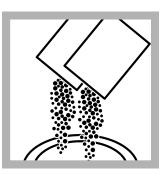
**3.** Add the contents of **one** PhosVer 3 HHC Phosphate Reagent Powder Pillow and **one** Ascorbic Acid Reagent Powder Pillow to the sample cell.
