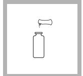
**4.** Add the contents of one NitriVer 2 Nitrite Reagent Powder Pillow, stopper and shake to dissolve (the prepared sample).
