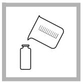
**6.** Fill another sample cell with 10 mL of sample (the blank). Place it into the cell holder.
