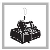
**9.** Place the prepared sample into the cell holder. Close the light shield. Results in mg/L NO<sub>2</sub><sup>-</sup> (or chosen units) will be displayed.
