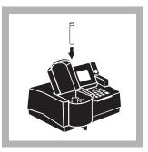
**12.** When the timer beeps, place the vial into the cell holder and close the light shield. The results in mg/L PO<sub>4</sub><sup>3-</sup> (or chosen units) will be displayed.
