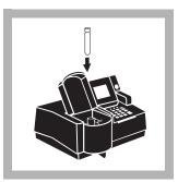
**6.** Place the vial into the cell holder and close the light shield.
