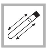
**9.** Cap the vial tightly and shake for 10-15 seconds.
