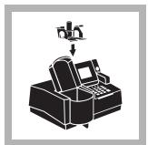
**4.** Insert the Test Tube Adapter into the sample cell module by sliding it under the thumb screw and into the alignment grooves. Fasten with the thumb screw.
