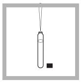
**3.** Use a TenSette Pipet to add 5.0 mL of sample to a Reactive Phosphorus Test 'N Tube Dilution Vial. Cap and mix.
