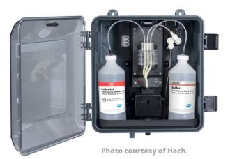
Figure 1. With automated operation and sufficient reagent storage, new ULR chlorine analyzers can provide precise readings of chlorine concentrations as low as to 8 ppb for up to a month in continuous production line operations.
