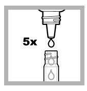
**9.** Immediately add **5** drops of Fluorescence Total Chlorine **Reagent 2**. Hold the bottle vertically.
