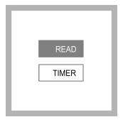
17. Select **READ**. The results show in ppb ( $\mu$ g/L). If the sample temperature is higher or lower than 20  $\pm$  3 °C (68  $\pm$  5 °F), refer to Temperature correction on page 4 to calculate the actual reading.
