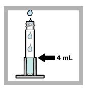
**7.** Put the sample vial in the sample vial holder. Add the sample to the top of the sample vial holder (4 mL).
