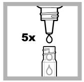
8. Immediately add 5 drops of Fluorescence Total Chlorine **Reagent 1**. Hold the bottle vertically.
