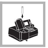
16. When the timer beeps, clean the outside of the Total Nitrogen Reagent C Vial containing the reagent blank. Place the vial in the adapter with the Hach logo facing the front of the instrument and close the light shield.
