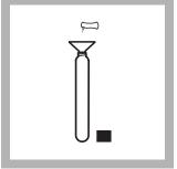
**10.** Add the contents of one Total Nitrogen Reagent A Powder Pillow to the vial containing the digested blank or sample. Cap the vial and shake for 15 seconds.
