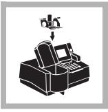
**15.** Insert the Test 'N Tube Adapter into the sample cell module by sliding it under the thumb screw and into the alignment grooves. Fasten with the thumb screw.
