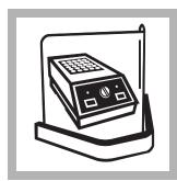
**1.** Turn on the COD Reactor. Heat to 103-106 °C (optimal temperature is 105 °C). Place the plastic shield in front of the reactor.
