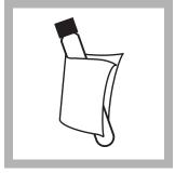
**18.** Wipe the Total Nitrogen Reagent C vial containing the sample.
