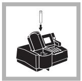
19. Place the vial into the cell holder with the Hach logo facing the front of the instrument and close the light shield. The result in mg/L total nitrogen will be displayed.
