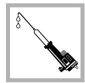
**3.** Hold the Digital Titrator with the cartridge tip up. Turn the delivery knob to eject air and a few drops of titrant. Reset the counter to zero and clean the tip.
