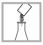
7. Add the contents of one Bromphenol Blue Indicator Powder Pillow. The indicator is not necessary if a pH meter is used.
