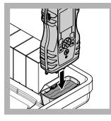
**5.** Put the meter into the sample cup.
